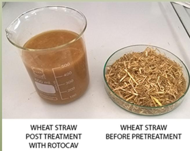
The pretreatment of the wheat straw with ROTOCAV ensured an increase in specific surface area, total pore and micropore volumes by a factor of 50%, compared to the wheat straw before the pretreatment.
